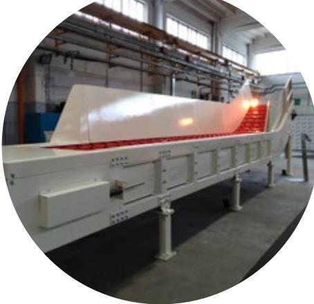
Aerothermic designed metal shutters, made from cold-bending, have a width either 1250 or 1500mm and a thickness of 5mm. The shutters are mounted on **the chain with bolts and locknuts**. On upper surface are mounted metallic pins in order to leave space between shutters and bales for **wires removal** after cutting.
