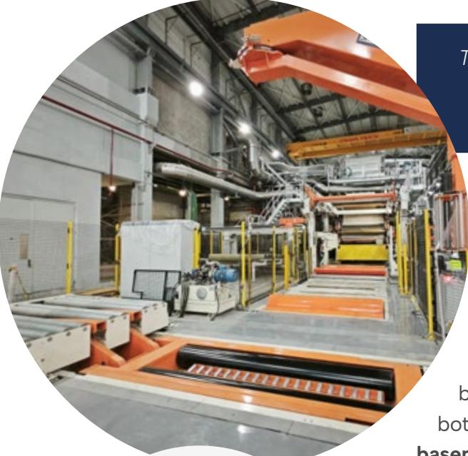
*The bottom part of the structure is ready for the installation of the film "cut and hold" group for the automatic management of the wrapping cycle (optional).*
