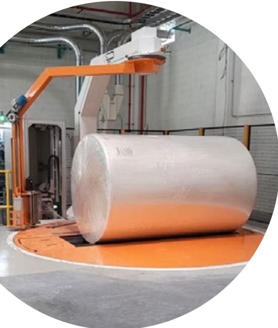
The structure which supports the rotating arm has a single column configuration and it contains every needed to move and to control the rotating arm. On **rotating arm** is installed a trolley which supports the film holder. The vertical trolley is moved in vertical position by means of a belt in order to vary the alignment of the stretch film reel with the center of the **paper reel to be wrapped**.
