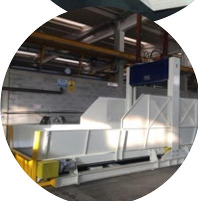
When the reel is positioned under the vertical portal, the Operator drives the **blade penetrates** the reel until you reach the inner cardboard core. The removal of the soul must be done manually by the Operator. When finished, the Operator may continue the descent of the blade in order to cut completely the resulting stack
